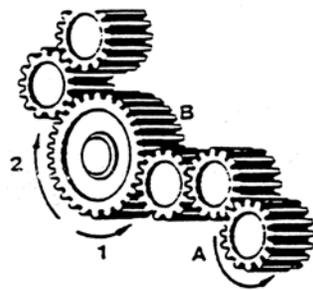
If cogwheel A rotates to the direction of the arrow, in what direction does cogwheel B rotate?
