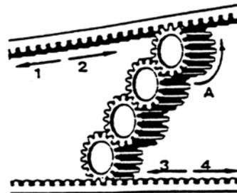
Cogwheel A turns to the direction of the arrow. In what direction do the cogwheels move?
