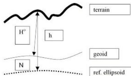
**Figure 3 – Orthometric and geodetic heights**
