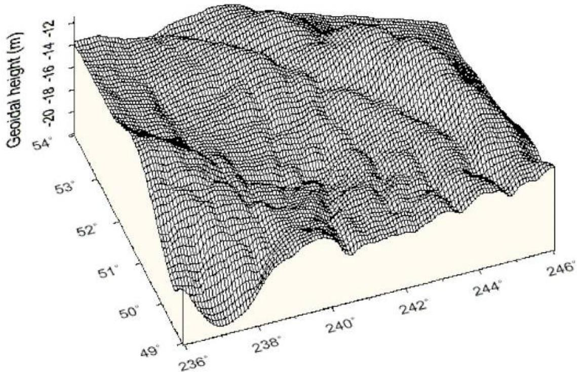
**Figure 11 – A 3D slice of the detailed geoid for North America (computed at the University of New Brunswick)**
