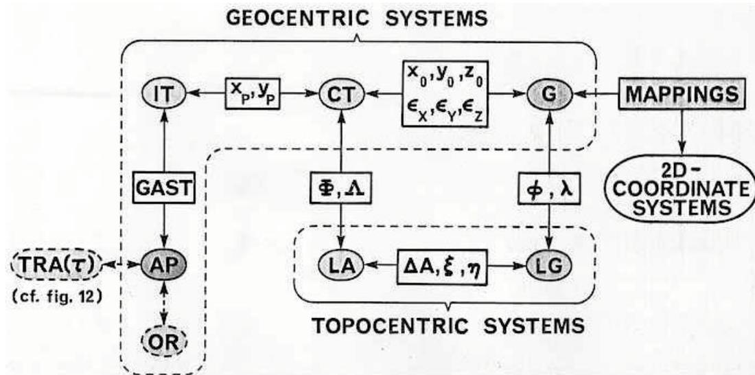
**Figure 8 – Commutative diagram of transformations between coordinate systems.**
