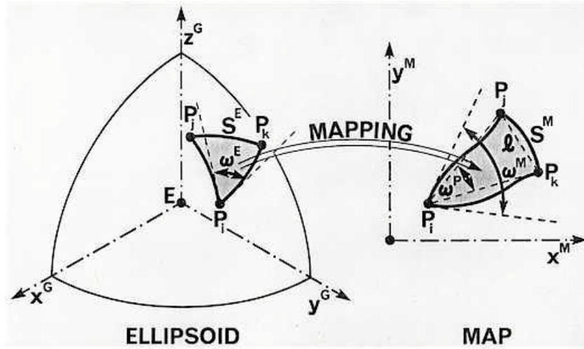
**Figure 4 – Mapping of ellipsoid onto a mapping plane.**
