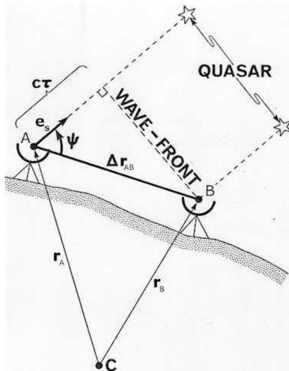
**Figure 5 – Radio-astronomical interferometry.**
