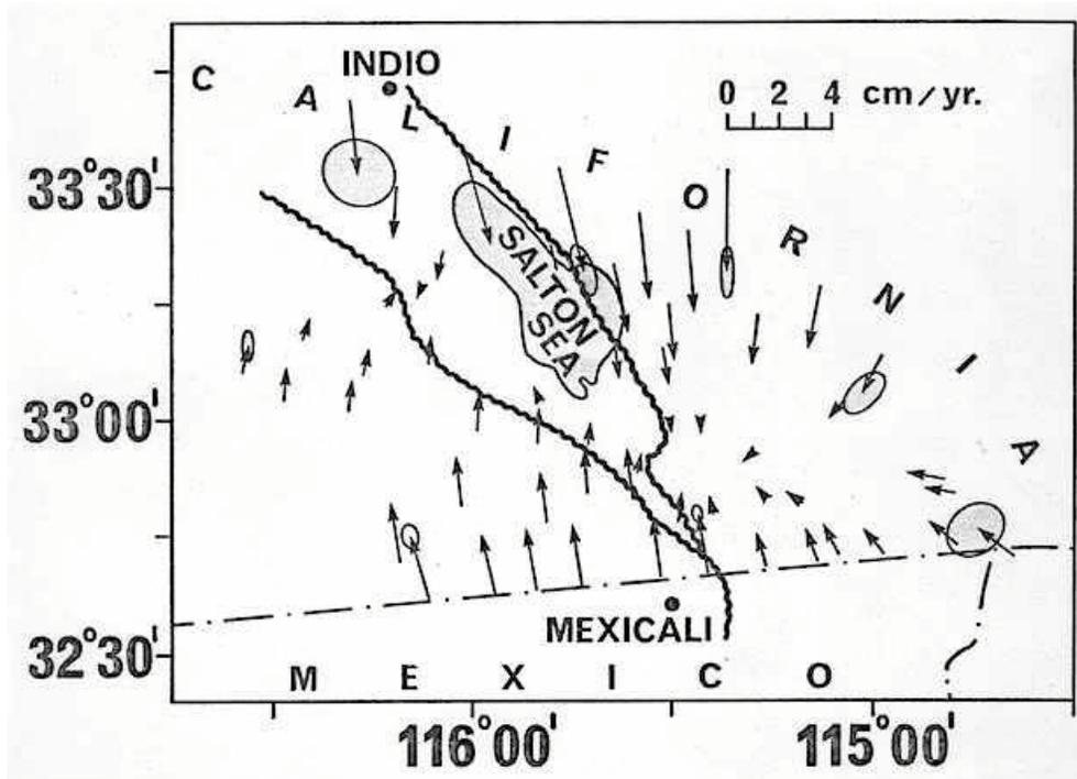
Figure 14 – Mean annual horizontal displacements in Imperial Valley, Cal., computed from data covering the period 1941 to 1975.
