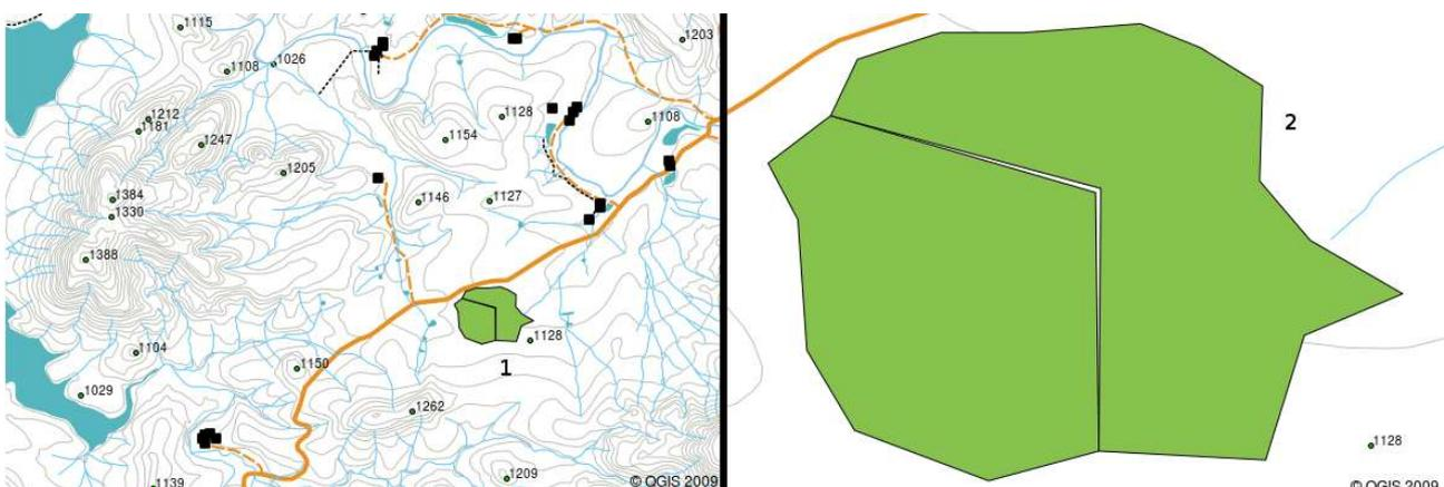
**Figure 16:** Undershoots (1) occur when digitised vector lines that should connect to each other don't quite touch. Overshoots (2) happen if a line ends beyond the line it should connect to.
